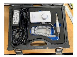
This micromotor is powered by a rechargeable control unit. The control unit is the white box on the top. That knob controls the speed of the tool. Jewelry burrs can be purchased from just about any jewelry equipment
